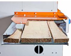
Max. width of workpiece: Unlimited. Max. edging width: 210 mm (8 5/16"). Max. thickness of the workpiece: 38 mm (1 1/2" Feed rate: 15 m/min\* (49 ft./min). Weight including machine stand: 240 kg (529 lbs). Electrical connection: 1-phase, 220 V, 30 A, 60 Hz.
