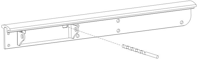
Drill instructions: Drill a 6 mm hole through the log bed. Normally, the log bed does not have to be detached from the sawmill. Overall view: Cross support
