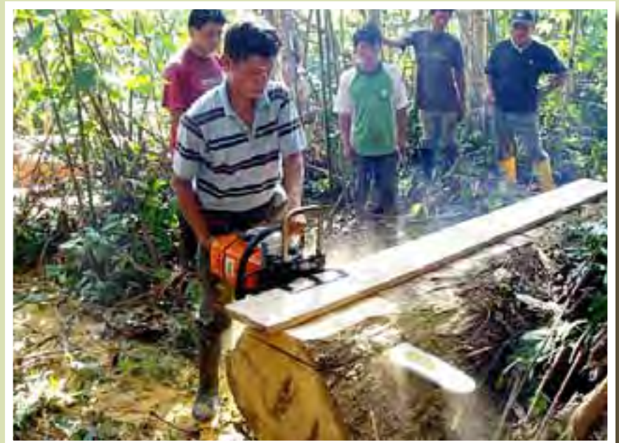
• A great combination: The TimberJig and a 36" picco bar and ripping chain making a test cut in Ecuador.
