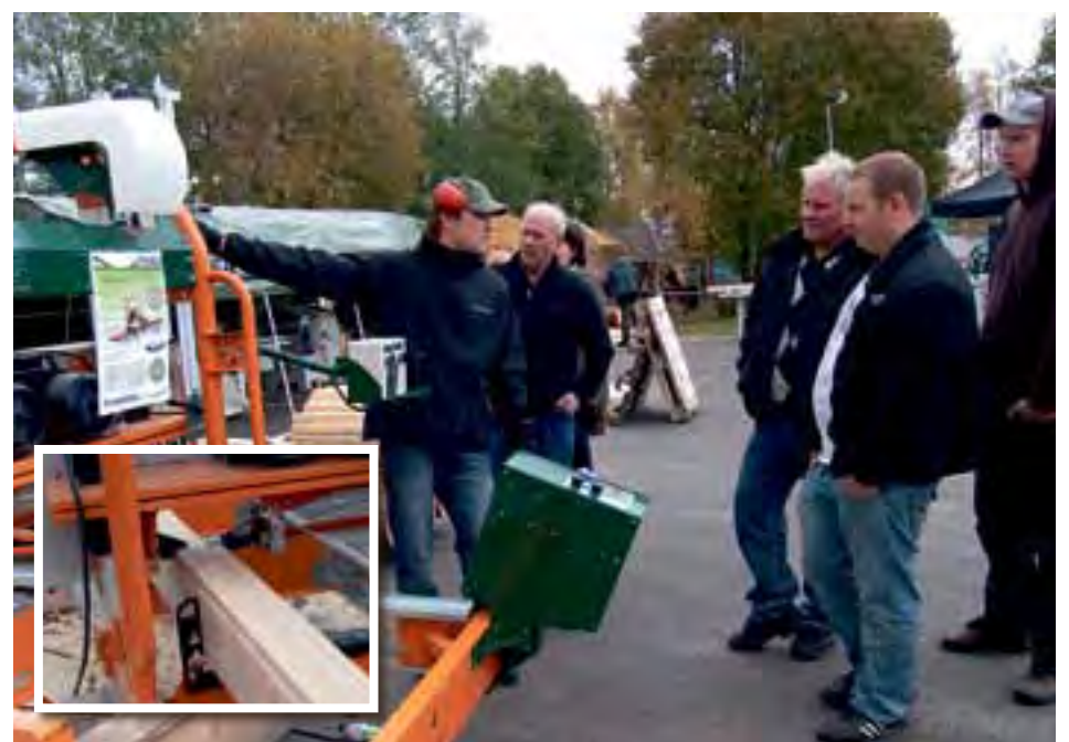
• Logosol's designer Jonas Höglund demonstrates the new feeder for the LM Pro bandsaw mill. Inserted image: Flaps that drop behind the sawblade.
