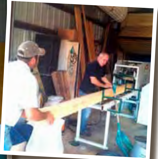
• Rusty and Kalle start a long leaf pine cant through the Logosol-LAKS Frame Saw in Louisiana.
