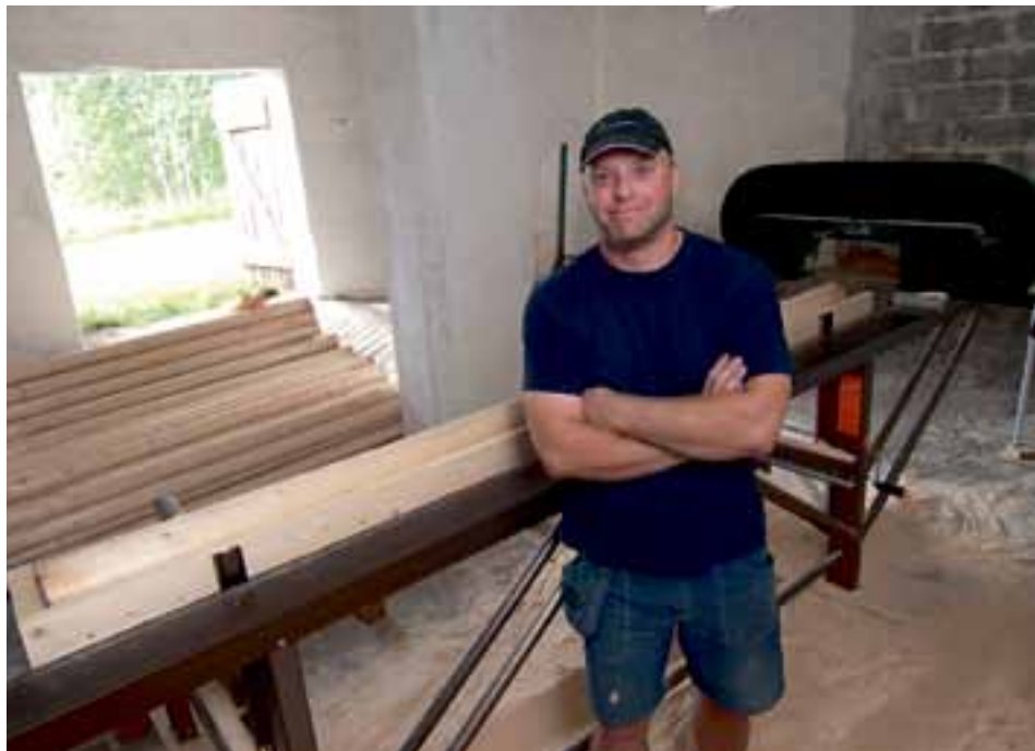
"It takes hardly any time at all to saw and the results are good," says Michael Högdahl, who makes shooting tower construction kits using a bandsaw on a Logosol sawmill.
